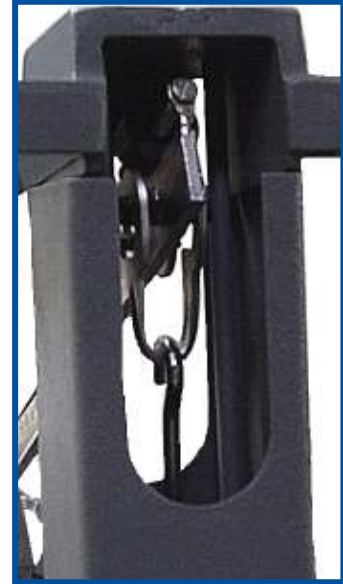
Hook the bottom Load Loop to the Steelyard Rod. Pulling the Beam up, hook the top Fulcrum Loop.
