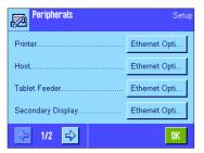
For each device only one connection can be made at the same time. It is for example not possible that two printers or two PCs can have a connection with the balance. A connection with more than one device (e.g. a PC with LabX and a LIMS System) is only possible when the balance is only activated as server (configurated as "open connection"). The devices must communicate temporary and after each other.
