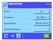
The parameters IP-address, Subnet Mask, Standard Gateway, Domain Name Server and Hostname are the (global) Network parameters for the Ethernet interface. Althought they are shown in every peripheral setting (Host, printer, second display, etc.), they are the same for each connection. These five parameters can only be set if the DHCP mode is switched off
