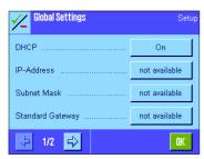
Using the ethernet set of protocols (TCP/IP), each machine that can connect to the ethernet needs a unique IP address. When a network of balances or other devices is set up, all devices must have an IP address be assigned to each one.
