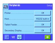
Select the desired peripheral with which the balance has to communicate over the Ethernet.
